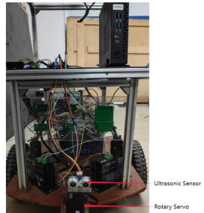
Figure 10 Experimental Robot
