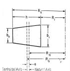
$$R_{N} = \frac{\left(\frac{b_{i} + b_{o}}{2}\right)h}{\left(\frac{b_{i} R_{o} - b_{o} R_{i}}{h}\right) \log_{e}\left(\frac{R_{o}}{R_{i}}\right) - (b_{i} - b_{o})}$$
